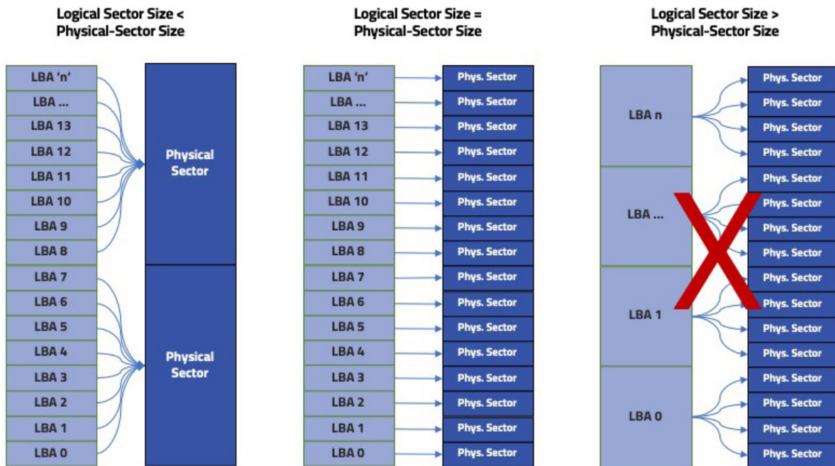
Figure 3: Logical to Physical-Sector Relationships
